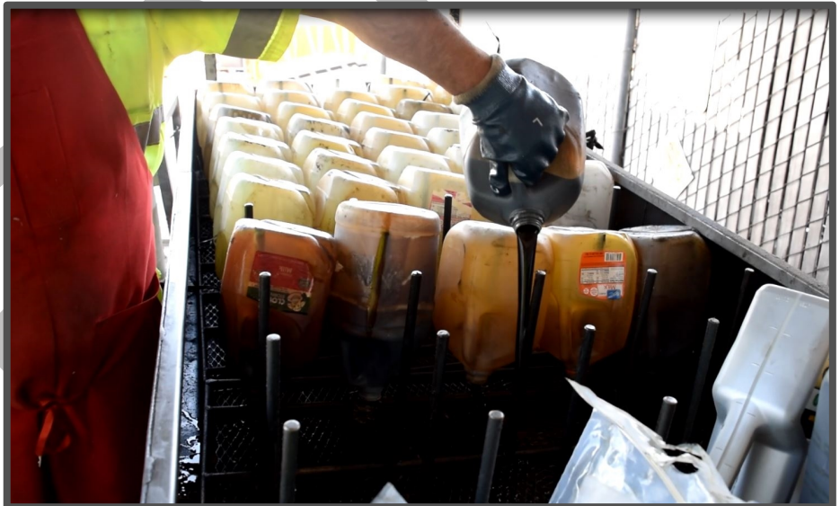
City of Vallejo Used Oil Transfer Station and Container Drain Rack Photo: Cal Poly San Luis Obispo
